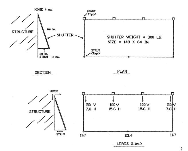
NDTE: The load at the hinge is vertically downward and horizontal away from the structure, and the load at the strut is horizontal against the structure. All loadings are Dead Loads only.
